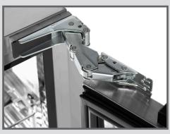
Heavy duty articulated hinges featuring soft self closing door. The hinge allows the door to open to 115° without touching adjoining cabinetry. (Decor panel max thickness is 19mm). Door is reversible
